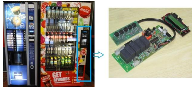
Figure 4: Beverage Vending Machine and its Embedded System. Source: (Park, 2006)
