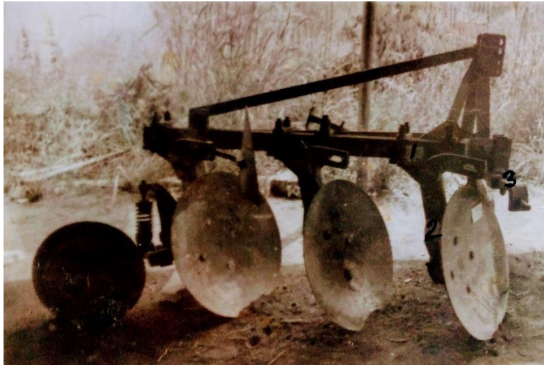
Figure 1: The 3-Bottom Disc Plough with adjustable Tilt and Disc Angles used for this work
