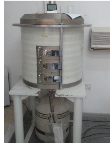
Plate 3. GEM 30195 detector mounted on 30-liter liquid nitrogen dewar for cooling to cryogenic temperatures and surrounded by lead shield to reduce the background caused by sources other than the sample.
