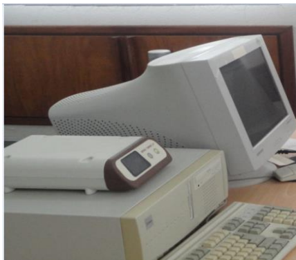
Plate 2. DSPEC jr 2.0 connected to desktop computer
